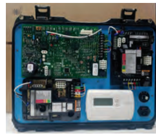
A customized PT-201 frame used for an OEM request.
