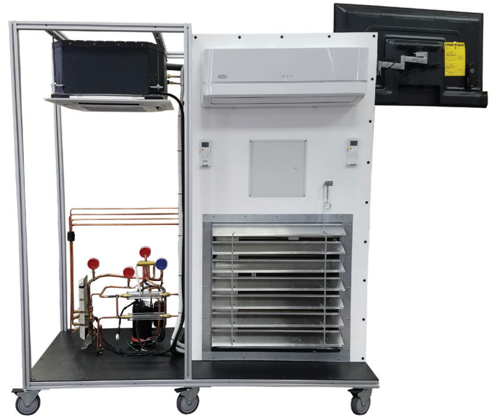
Back side of unit showing louvers and wall-mounted unit
