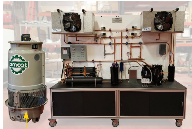
OPTIONAL WATER TOWER AND WATER PUMP
